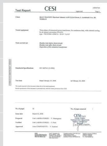
630KVA, 20/0.4kV Power Transformer Type and Short-Circuit Tests CESI Lab.
